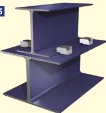
Drilled I-Section running parallel to another I-Section
