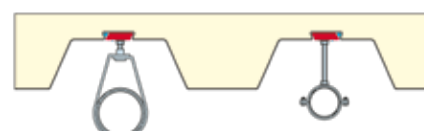
Typical pipe supports
