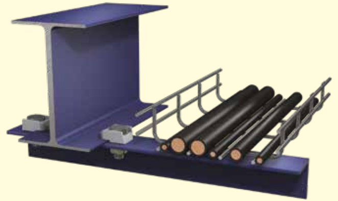
Cantilevered angle support for running cable tray
