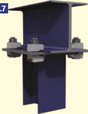
I-Section to top of a column end plate
